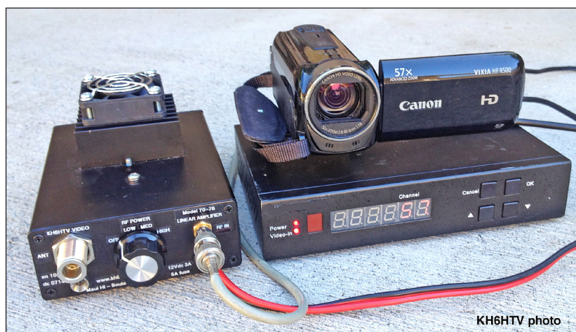
Figure 11 — The author’s ATV transmitter system consists of a Hi-Des HV-320E DVB-T modulator driving a KH6HTV 70-7B linear amplifier for the 70 cm band. The modulator also tunes the 33, 23, and 13 cm bands and has an adjustable output up to 6.5 dBm on 70 cm.
