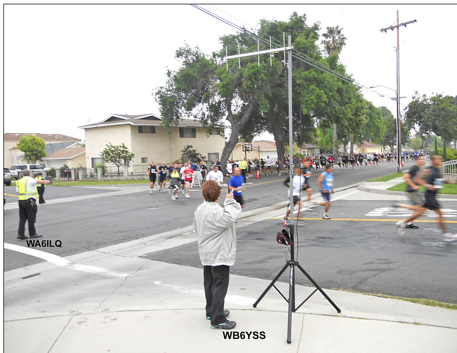
Figure 2 — A low power 70 cm ATV transmitter can be used to show conditions on a racecourse or at aid stations. This setup delivered video over a 2-mile path.
