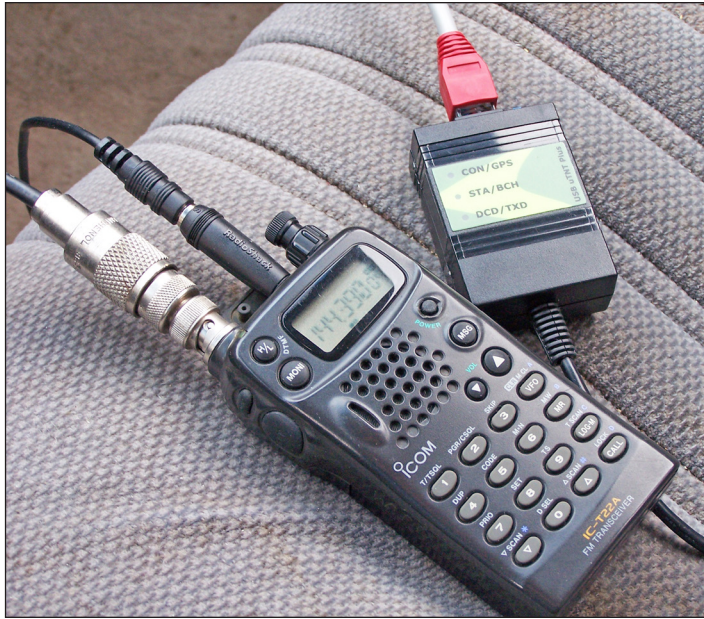
Figure 6 — A 2-meter FM handheld trans- ceiver attached to an APRS position encoder.
