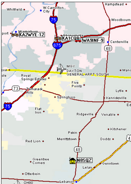
Figure 7 — A snapshot of APRS activity using UI-View software. Note the icons representing various mobile and fixed stations.
