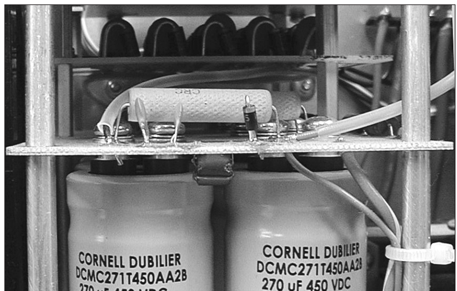
Figure 7.45 — Example of the filter capacitor/bleeder resistor installation in a high voltage power supply.
