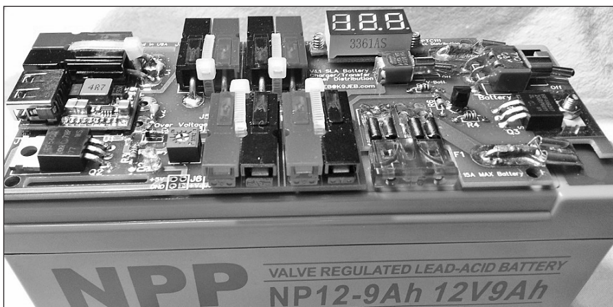
Figure 7.64 — The charging circuit shown mounted directly on a 9 Ah SLA battery. Note the USB charging module mounted next to J1 at the left-hand side of the board.
