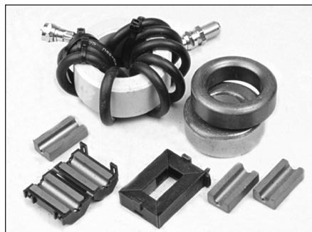
Figure 27.12 — A common-mode RF choke wound on a toroid core is shown at top left. Several styles of ferrite cores for common-mode chokes are also shown.
