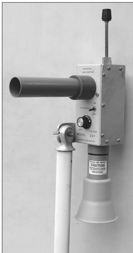
Figure 27.37 — The Radar Engineers Model 247 Hotstick Line Sniffer is an RF and ultrasonic locator. It is used by utility workers to pinpoint the exact piece of hardware causing a noise problem.
