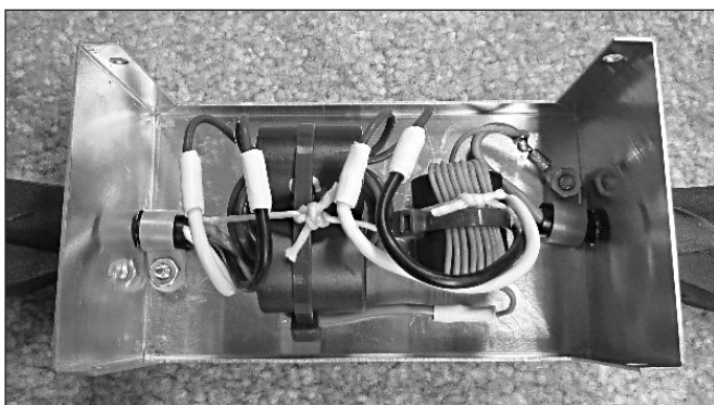
Figure 27.33 — Common-mode filter for electronic lighting ballast, designed and built by Tom Thompson, W0IVJ.
