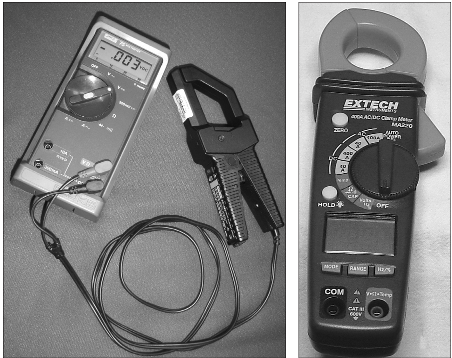
Figure 26.2 — A clamp-on meter probe is used with a digital multimeter for measuring ac current (left). Meters are also available integrated with the clamp-on probe (right).
