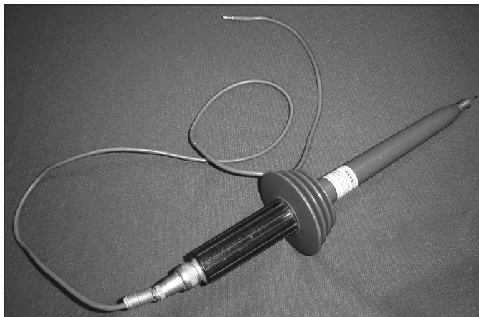
Figure 26.3 — A probe used for measuring high-voltage with a standard multimeter.
