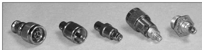
Figure 25.32 — Coaxial connector adapters. From the left are: BNC male to type-N male, BNC female to UHF male, BNC female to SMA male, type-N male to SMA female, and type-N female to SMC male.
