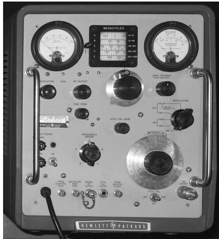
Figure 25.9 — A classic Hewlett-Packard 608F tube-type signal generator. While not as stable as modern synthesized signal generators, in other respects the performance is quite up to date.
