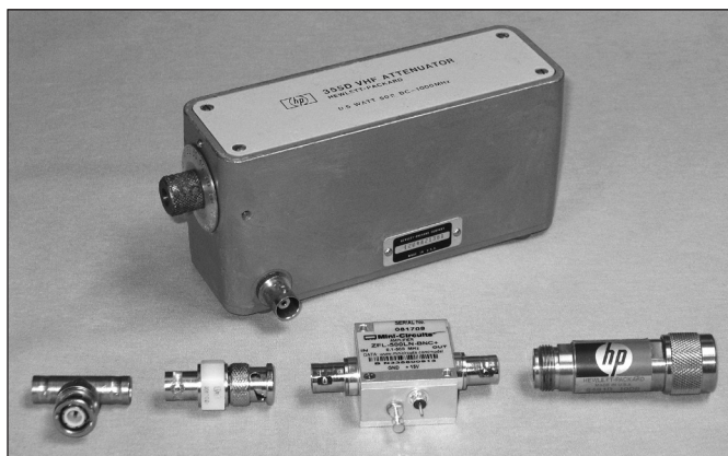
Figure 25.31 — Various RF test accessories. At the rear is a 10 dB step attenuator with a 0-120 dB range. In the foreground from left to right are a BNC “T” connector, a 50- \Omega feed-through termination, a 0.1-500 MHz low-noise amplifier, and a 10-dB fixed attenuator.
