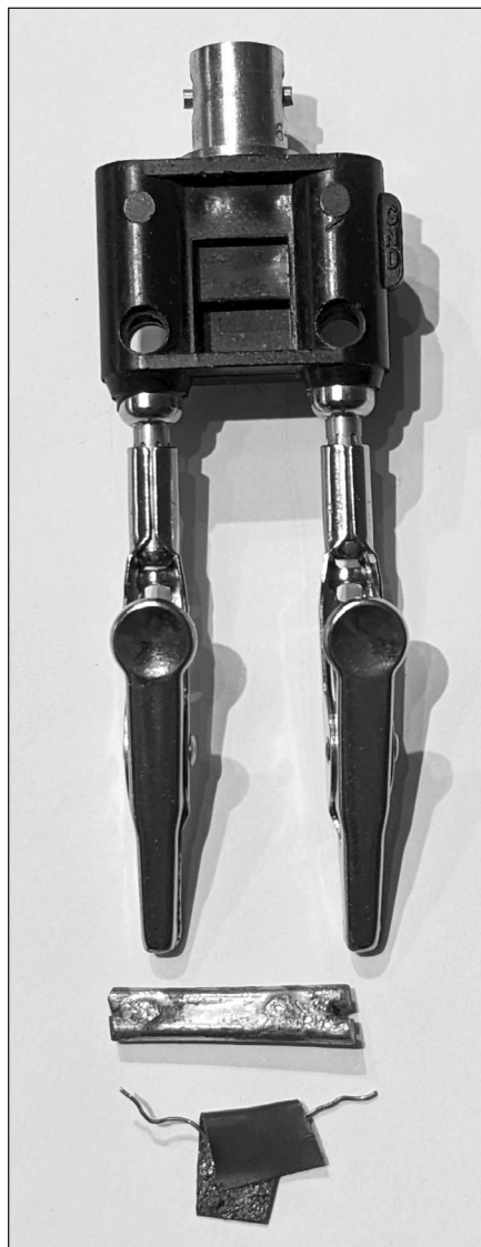
Figure 25.28 — A simple vector impedance analyzer (VIA) test fixture for measuring component impedance into the VHF range. The fixture is a BNC-to-banana plug adaptor with alligator clips on the plugs. Below the clips are the short-circuit calibration load and a non-inductive 50- \Omega resistor to perform the SOL calibration. (Photo courtesy of Jim Brown, K9YC)
