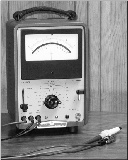
Figure 25.4 — This classic Hewlett-Packard HP412A vacuum-tube voltmeter (VTVM) has specifications that put many modern solid-state multimeters to shame.
