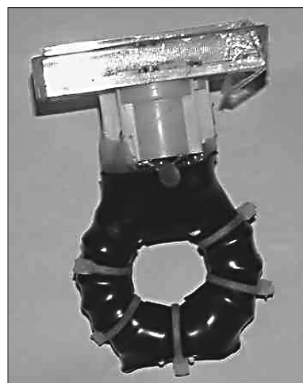
Figure 25.75 — Assembly of the RF current probe. Use an all-plastic meter and mount the circuits and toroid directly on the back of the meter case.
