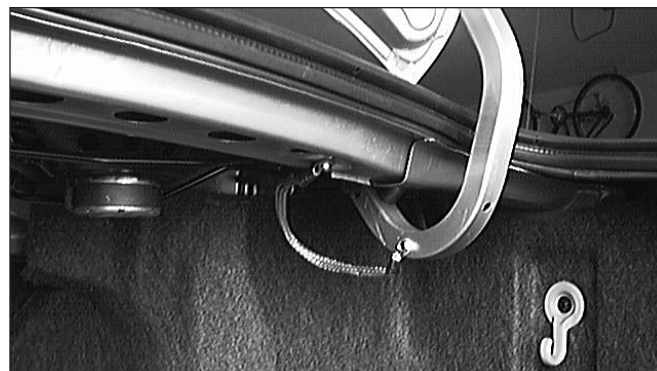
Figure 24.29 — Bonding vehicles parts — in this case, the trunk lid to the main body — can help reduce interference.
