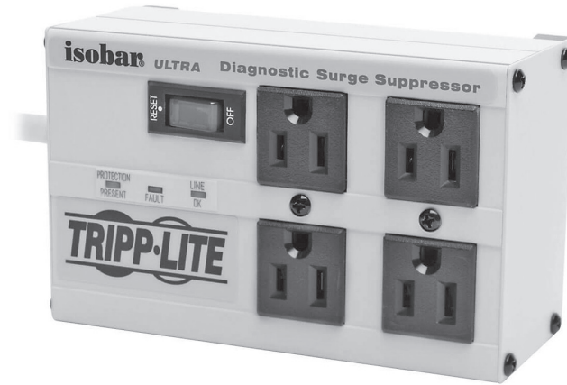
Figure 24.7 — An in-line ac power line surge protector suitable for lightning protection. It may be connected to a grounded panel via one of the enclosure screws.
