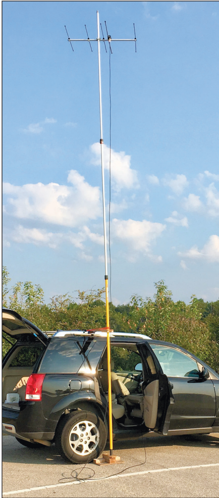
Figure 24.35 — The K5ND/r push-up mast (a painter's pole) on a drive-on base with a stabilizing brace attached to the roof rack.
