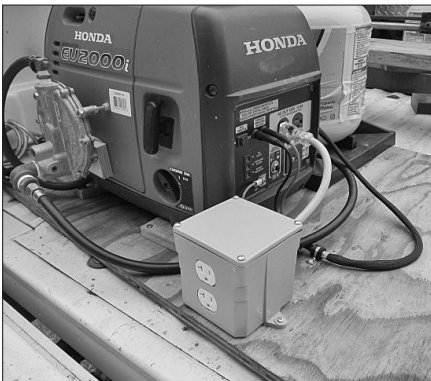
Figure 24.33 — A heavy-duty common-mode RF choke wound on Type 31 ferrite cores for ac generators. K9YC and W6GJB use this choke during portable operating. See the text for construction details.
