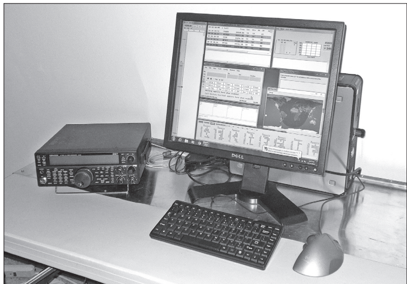
Figure 24.9 — A simple RF ground plane made of aluminum roof flashing with a copper pipe bonding bus attached at the rear of the table. Equipment is placed on the flashing and attached to the pipe with short jumpers. The ground plane and bus are attached to the station ground system with a heavy wire. [Ward Silver, NØAX, photo]
