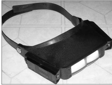
Figure 23.5 — A magnifying visor is great for close-up work on a circuit board. These headsets are often available for less than $10 at hamfests, and some even come with superbright LEDs mounted on the side to illuminate the components being soldered.
