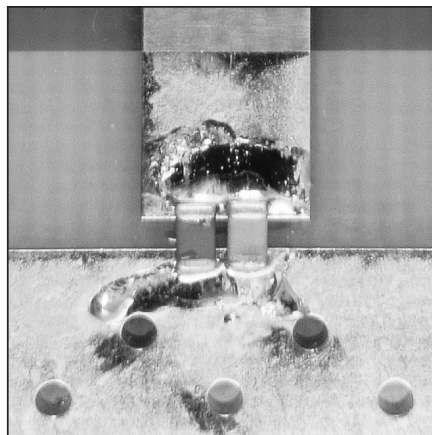
Figure 23.36 — Printed comb-line filter uses two chip capacitors in parallel to reduce loss.
