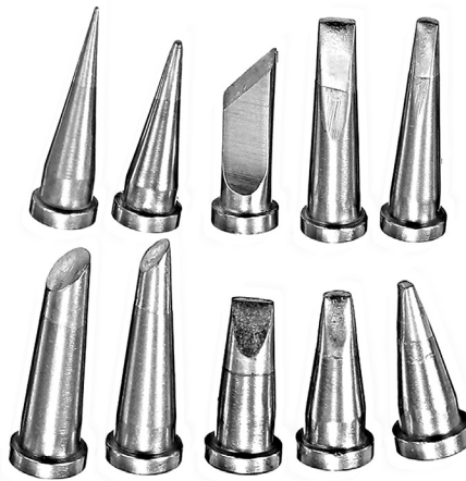
Figure 23.2—Typical soldering iron tips (this group is from Weller, weller-tools.com ). Conical tips are shown at the upper left and chisel tips at the upper right. Larger connections require the heavier tips.
