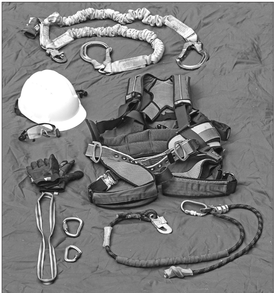
Figure 22.19 — Typical climbing equipment. From the top and left to-right, fall arrest lanyards with "gorilla hooks," hard hat and safety glasses, body harness, gloves, nylon sling, carabiners, and positioning lanyard. (Jim Idelson, K1IR, photo)
