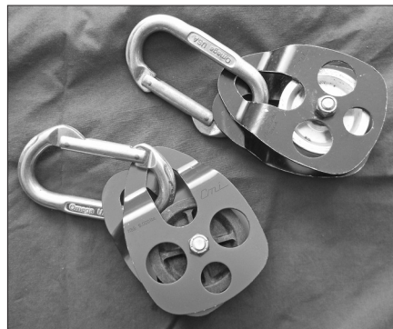
Figure 22.15 — Snatch blocks can be opened to place a rope directly on the sheave without having to thread it through the housing. A lightweight plastic block is shown at left, and two metal housing blocks at right.
