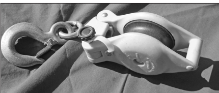
Figure 22.15 — Snatch blocks can be opened to place a rope directly on the sheave without having to thread it through the housing. A lightweight plastic block is shown at left, and two metal housing blocks at right.
