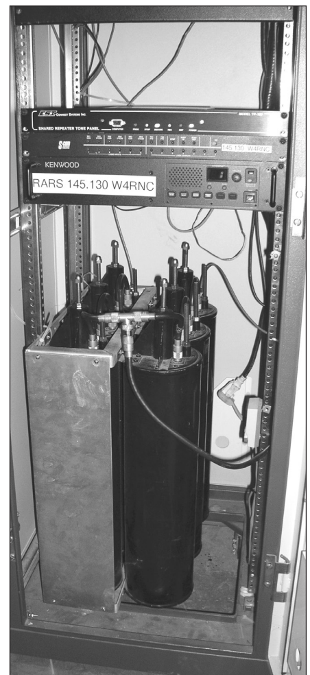
Figure 18.6 — The W4RNC 2 meter repeater includes the repeater receiver, transmitter, and controller in the rack. The large object underneath is the duplexer. [Photo courtesy Gary Pearce, KN4AQ]
