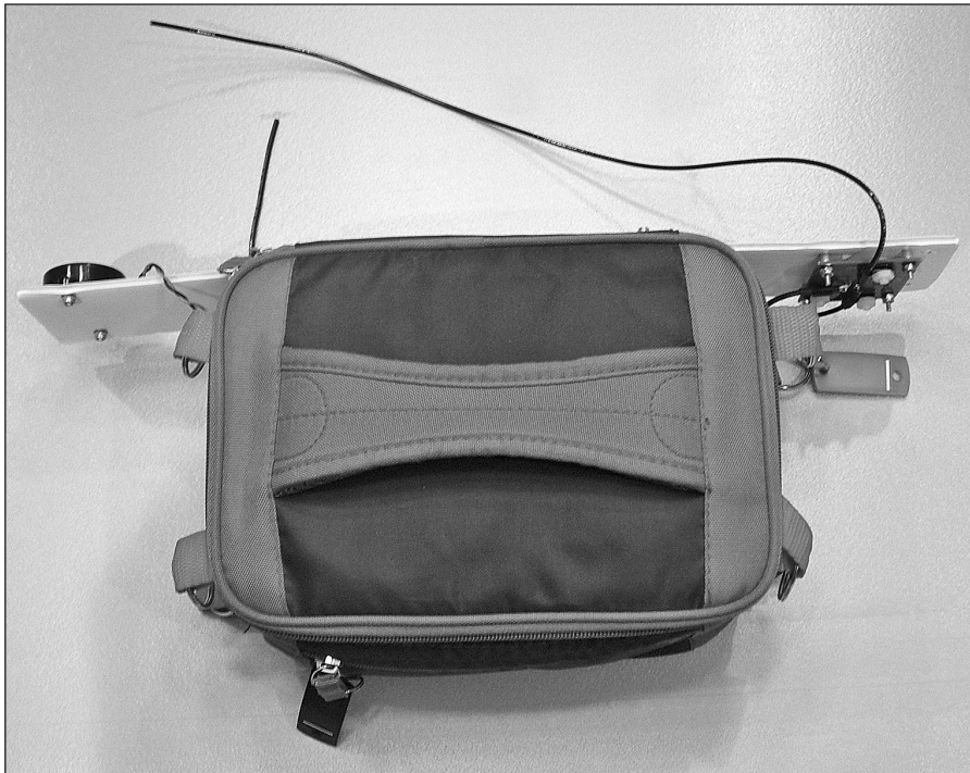
Figure 16.13 — The complete Near Space Tracker assembled in an insulated fabric lunch cooler.
