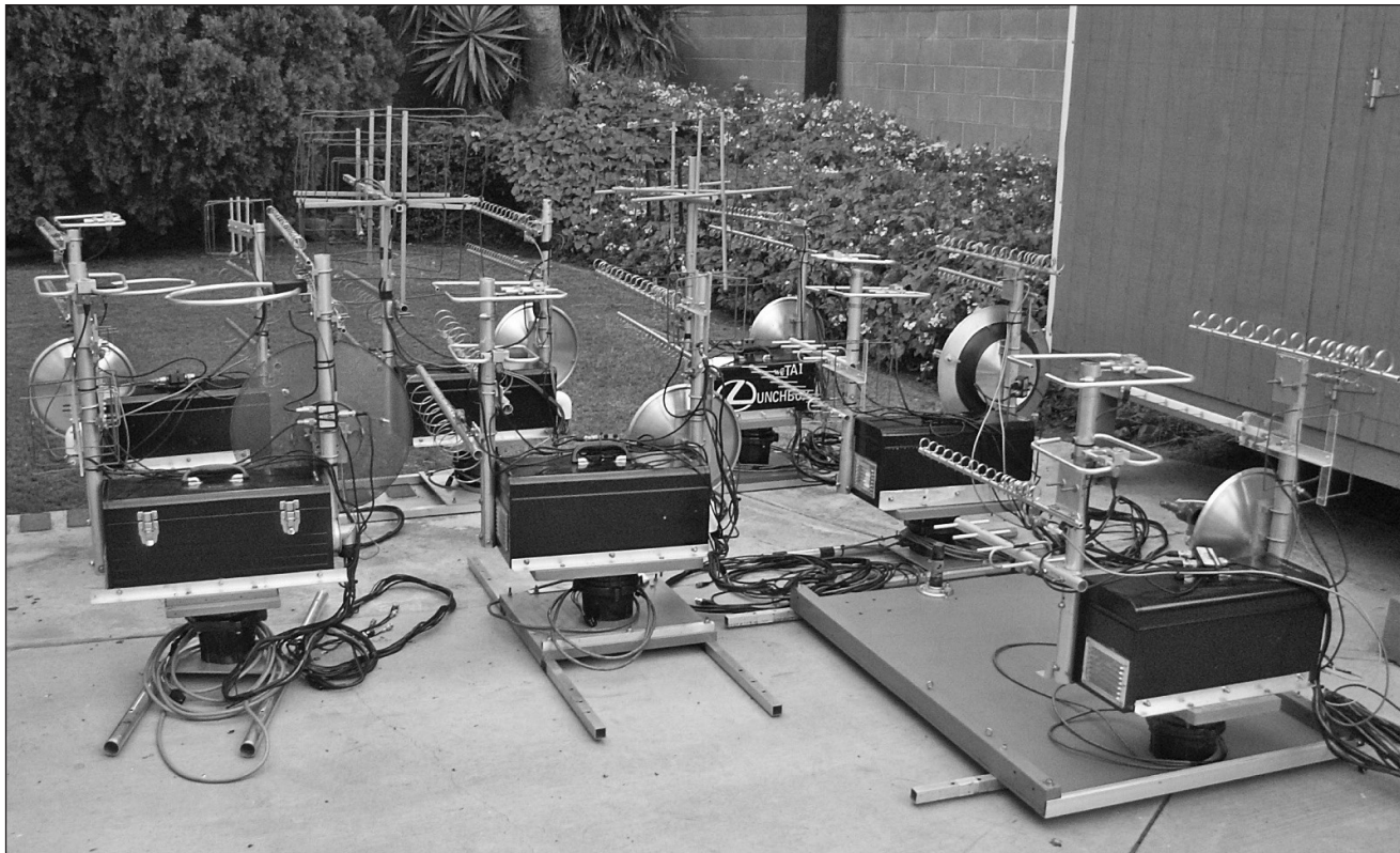
Figure 14.28 — Seven transverter packages designed to be mounted on the roof of the vehicle with antennas attached.
