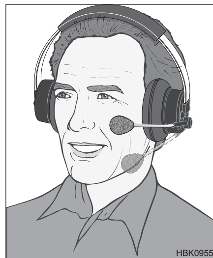
Figure 13.48 — Using a computer-style headset electret boom microphone. Place the microphone far enough from your mouth to avoid picking up excessive noise from breathing and pops from speech. Balance the placement for normal speech levels while minimizing pickup of room and fan noise. On-the-air testing is important to account for your station circumstances and speaking style.
