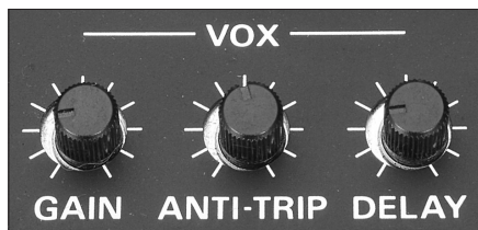
Figure 13.62 — The function of VOX controls is described in the text. They require adjustment for different types of operating, so front-panel knobs make the most convenient control arrangement. In some radios, VOX settings are adjusted through the menu system.
