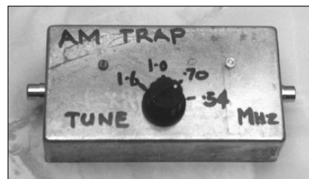
Figure 10.84 — The wave trap can be roughly calibrated to indicate the frequency to which it is tuned.
