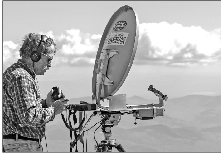
Figure 1.10 — Amateur radio frequency allocations extend well into the microwaves. Here, Chip Taylor, W1AIM, hunts contacts on the 10 GHz band from Mount Washington in New Hampshire, some 6,200 feet above sea level. [Chris Craig, K1MHZ, photo]
