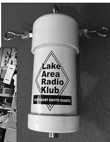
Figure 1.8 — Antennas are always a popular topic among hams. The Lake Area Radio Klub (LARK) in South Dakota embarked on a club project to design and build baluns for use with wire dipole antennas. It offered club members a chance to learn more about antennas and build a useful project for their station. Rich Grant, KE0EPY, helped club members with assembly.
