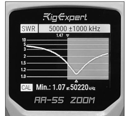
Figure 1.11 — Learning to use basic test equipment such as an antenna analyzer will help you keep your amateur station running at peak efficiency,
