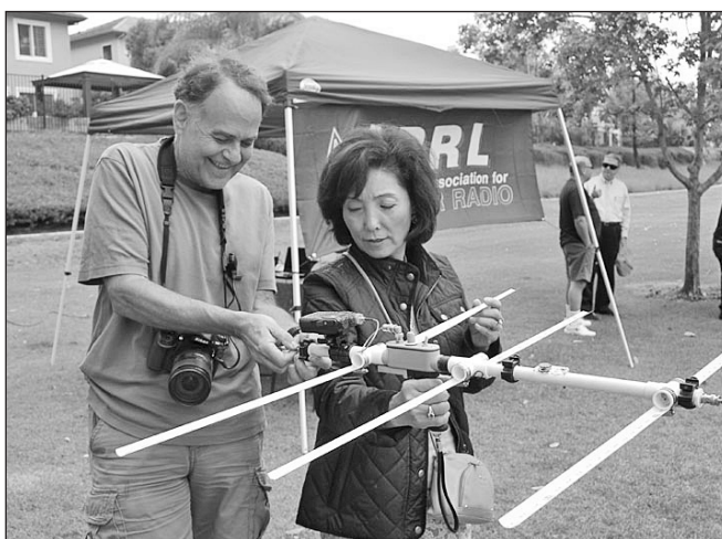
Figure 1.22 — Amateur Radio Direction Finding (ARDF) equipment need not be expensive. Yagis made from measuring tapes and PVC pipe are very popular for direction finding on 2 meters with a handheld transceiver. Here, Dan Slater, AG6HF (left), tests an antenna he built. [Joe Moell, K0OV, photo]
