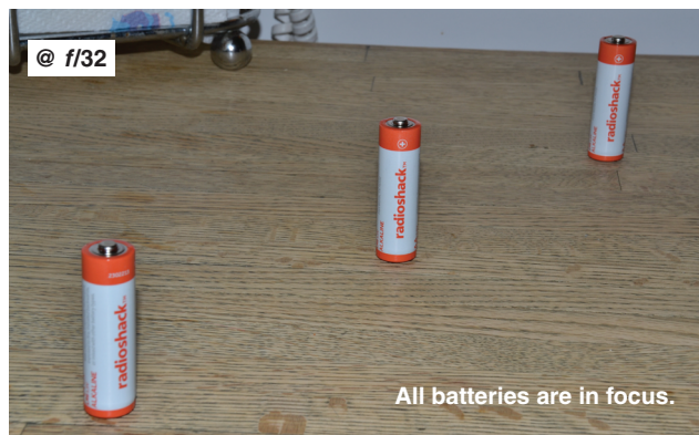
Figure Q-7 Reduced depth of field in images obtained with lenticular optics. Even in this case, smaller apertures (larger f /numbers) result in greater depth of field. (Courtesy of Scott E. Brodie, MD, PhD.)
