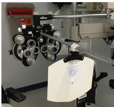
Figure Q-31 Phoropter with near-point chart in place, 40 cm away. (Courtesy of Scott E. Brodie, MD, PhD.)
