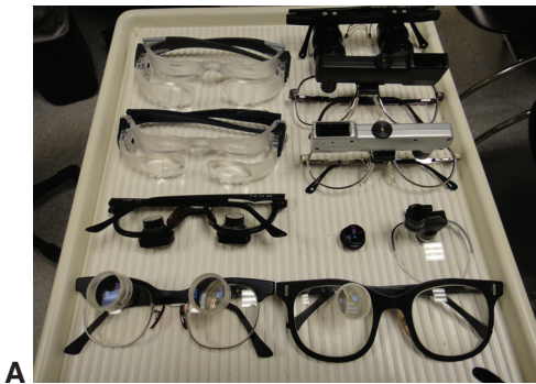
Figures 10-11 Telescopic devices. A , The range of telescopic devices includes monocular and binocular telescopes. B , This binocular spectacle telescope is lightweight and can be used for stationary distance viewing such as watching television. (Courtesy of Mary Lou Jackson, MD.)
