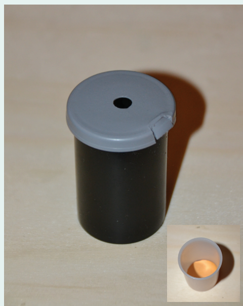
Figure Q-34 Film cannister modified for use as a model eye for retinoscopy practice. The hole punched in the lid should be about 5–6 mm in diameter; it is helpful to tape an orange disk of paper at the bottom of the canister ( inset ) to create more realistic reflexes. (Courtesy of Scott E. Brodie, MD, PhD.)
