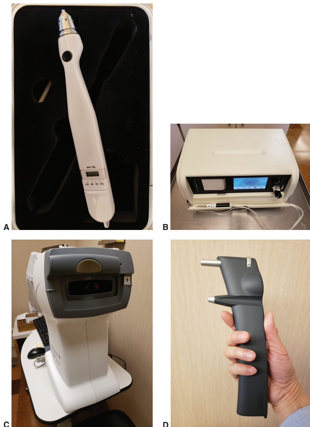
Figure 2-7 Nonapplanation tonometers in common use offer advantages and disadvantages compared with Goldmann applanation tonometry. A , Tono-Pen. B , Pneumatonometer. C , Ocular Response Analyzer. D , Rebound tonometer. (Courtesy of Arthur J. Sit, MD.)
