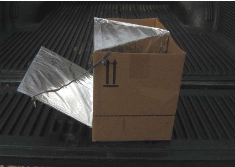
Side view showing the adjustable front panel and the string used to hold the panel in the desired position.
